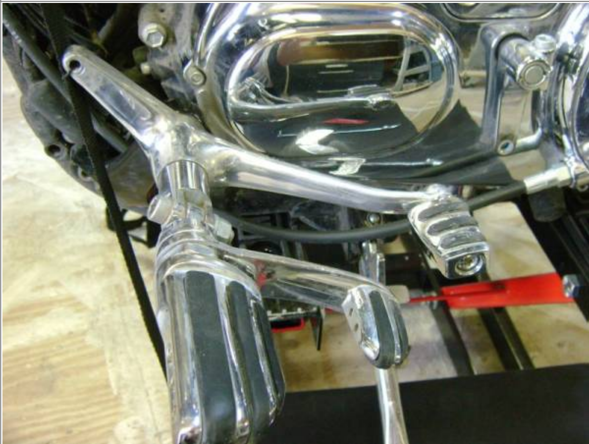
The shift lever assembly has been rotated clockwise 180 degrees
