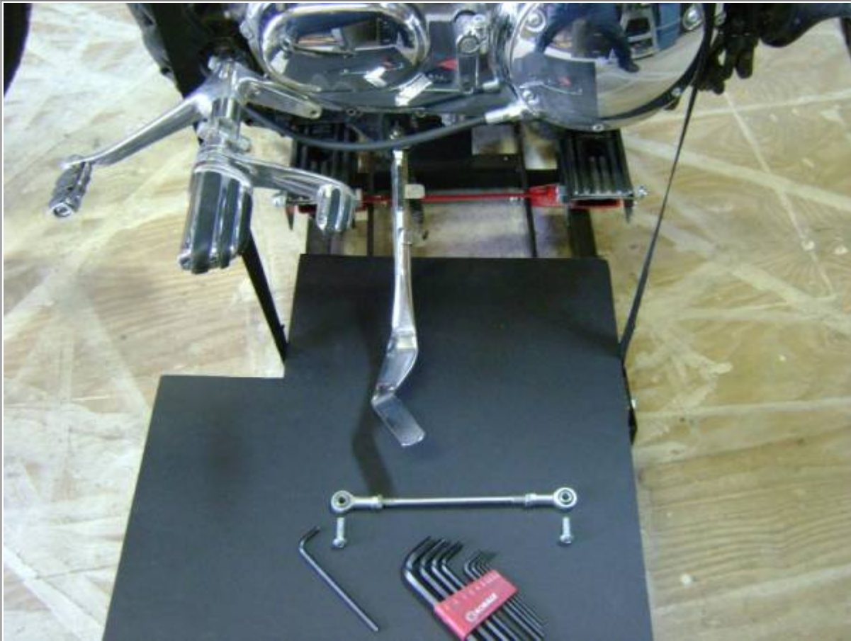
The shift lever assembly has been rotated clockwise 180 degrees
