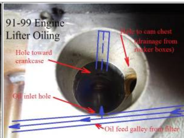
A look inside the oiling holes in the lifter bore on a 91-99 case. Notice the capped hole toward the case in the third pic. 41)
