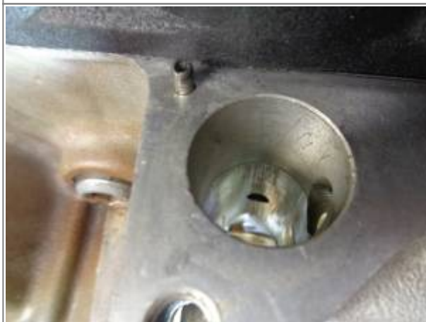
A look inside the oiling holes in the lifter bore on a 91-99 case. Notice the capped hole toward the case in the third pic. 41)
