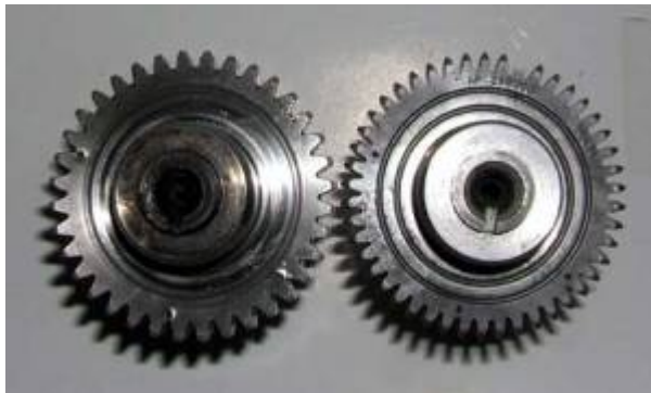
1991-1999 cams (left) have a coarse tooth pitch. 2001-up cams (right) have a finer tooth pitch referred to as High Contact Ratio (HCR). 2000 model cams have HCR on the pinion connection only, and the 91-99 style coarse tooth pitch for all other connections.
