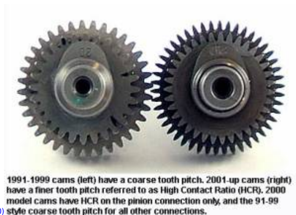
1991-1999 cams (left) have a coarse tooth pitch. 2001-up cams (right) have a finer tooth pitch referred to as High Contact Ratio (HCR). 2000 model cams have HCR on the pinion connection only, and the 91-99 style coarse tooth pitch for all other connections.
