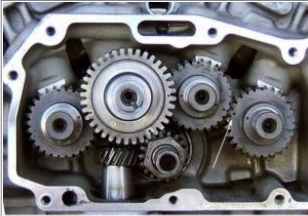
This picture shows proper alignment of the cam marks. Be sure you have the mark that's pointed to by the arrow. If it's not there, double check to make sure you haven't swapped the number 1 and 4 cams by mistake.
