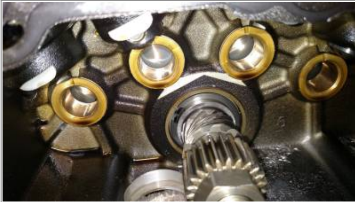
2010 1200X Inner Cam Bushings (broken teeth on oil pump gear) 24)
