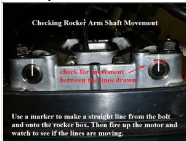
Checking rocker arm shaft movement 1)
