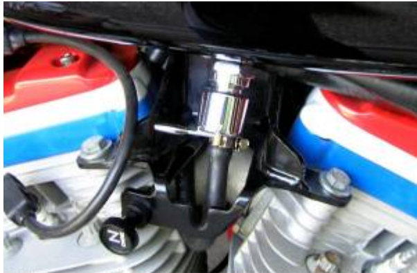
1994 Sportster with 1997 Custom fuel tank, (3.3 gal, left side petcock), using a 1998-2003 top center motor mount bracket
