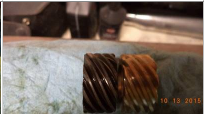
Comparison with a new bronze gear. 53)
