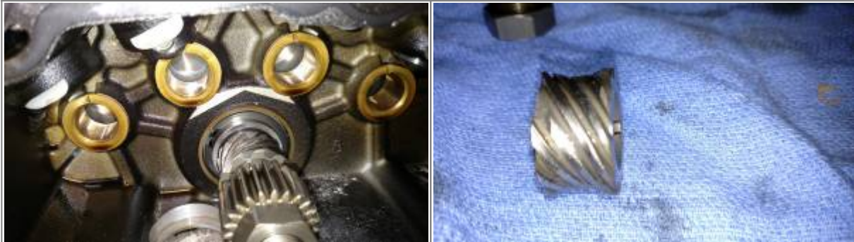
More oil pump and drive gear damage 56)
