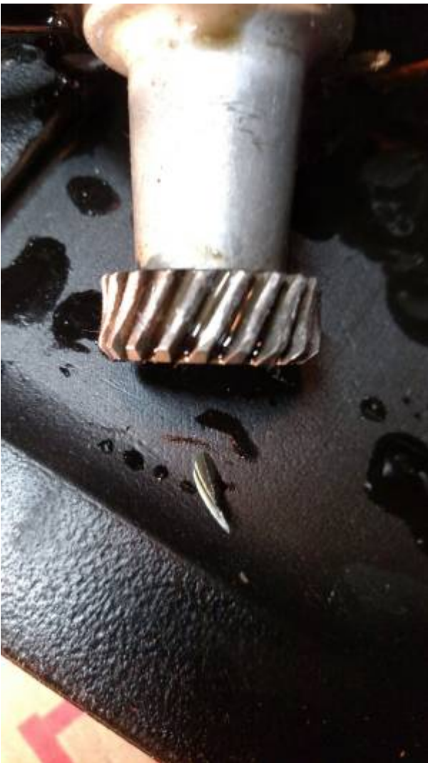
A chunk of a tooth from the oil pump gear fell out of the oil
