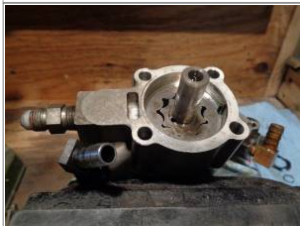
Return (scavenge) gerotors installed position 17)
