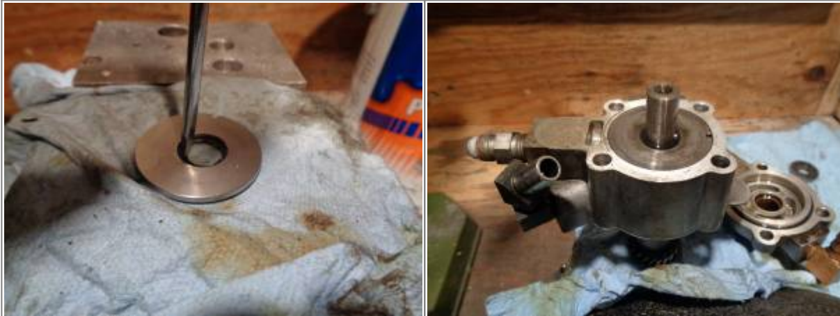
Outer seal (12036A) installed position. 9)
