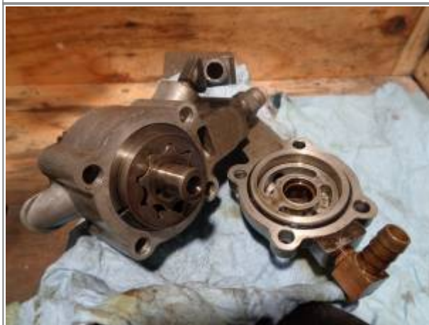
Feed gerotors installed location 15)
