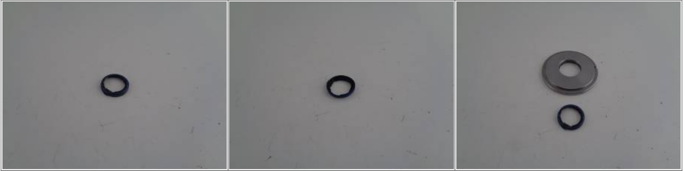
Outer plate seal (12036A) (destroyed during removal) 8)
