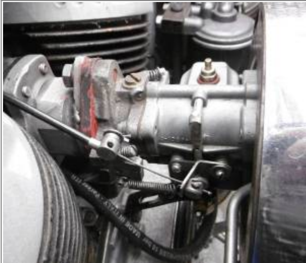
Linkage modified for usage with "snap" throttle 17)
