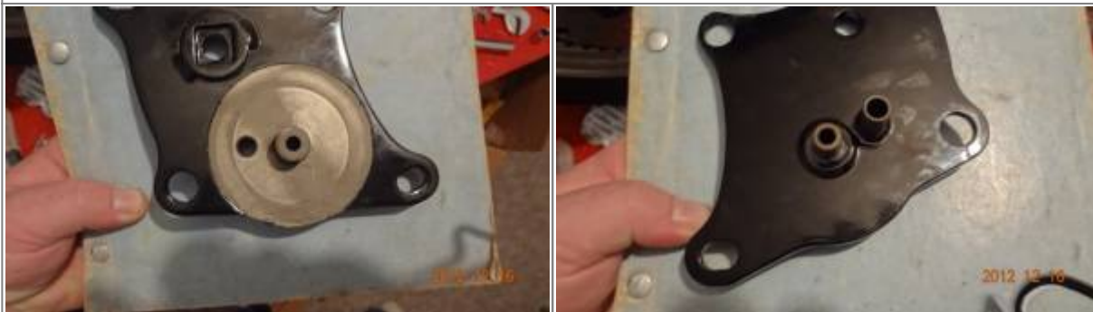
82-E84 lower front motor mount / filter mount. 56)
