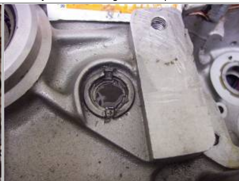
The transfer below valve below was packed with JB Weld to negate it's operation. 6)
