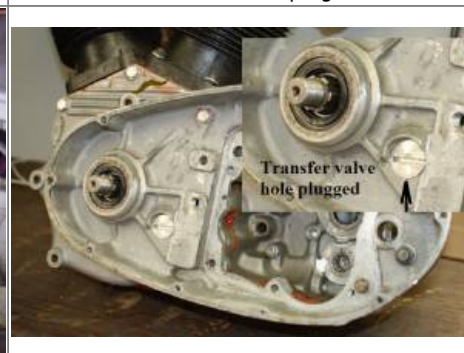
Transfer valve removed, plug installed. 7)
