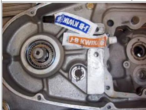
The transfer below valve below was packed with JB Weld to negate it's operation. 6)
