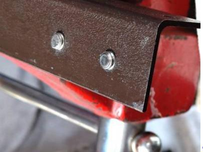
The outer pad and rivets are positioned on the floating pad plate and set on the jig. The rivets are hollow. A tapered center punch was used first to flare the tips. Then a flat 5/16" punch was used to flatten and secure the rivets and pad. Be careful not to over-tighten and crack the pad.
