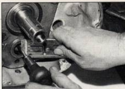
31 The correct way to check the end play of the countershaft (.004" - .009") is with a dial indicator. But if you don't have one, see the sidebar "End Play Checks" to see how you can get it close, or on, using a razor blade and feeler gauge.
