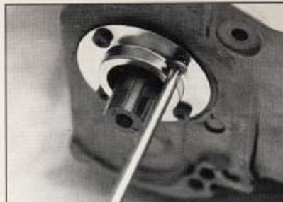
34 The last parts to go on are the oil seal and retainer, which can be purchased as a set (H-D #35150-52), and its gasket (H-D #35169-52). Clean off the gasket surface and install these with four screws (H-D #2669W) and lock washers (H-D #7025W).
