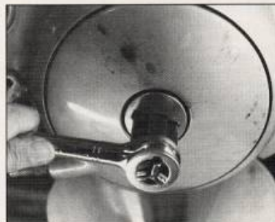
5 The old 'Chevy tool' is used to remove the clutch adjuster plug.
