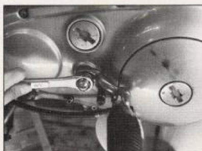
3 Then you can remove the shift lever and footpeg.
