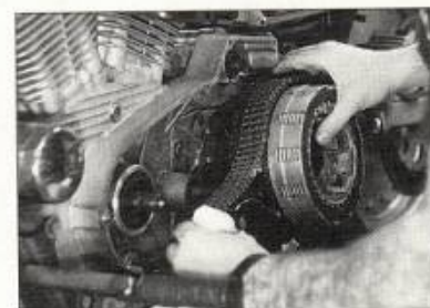
6 After removing the engine sprocket, Rich can remove the entire primary drive and clutch at the same time.
