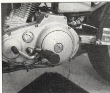
1 First things first; before placing my Sportster on a lift, Rich drains the primary/transmission oil.
