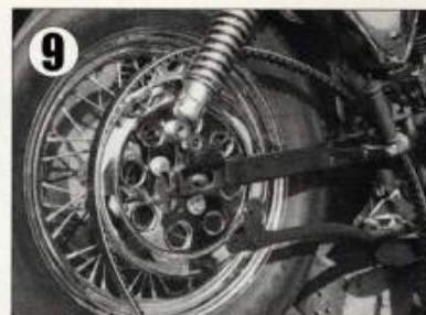
9 Place the belt over the rear pulley and, with your buddy helping, lift the wheel into place. Coat the axle with anti-seize and push it through from the left side of the swingarm. Install the washer and nut, hand tight only. Then drape the belt over the tranny pulley.
