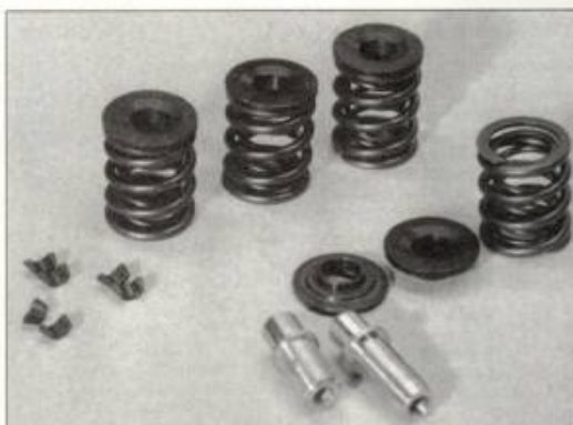
These springs (two per set), upper collars (on top of three of the spring sets), valve locks (two per valve), and guides (only one exhaust and one intake is shown) are all Manley components. The lower collars (one is showing with the others under the spring sets) are H-D units. Manley does not send lower collars with the kit because the stock units work fine.
