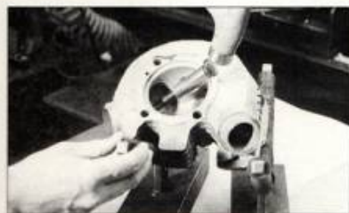
Machinist Bob Sommer removes the old valve guides using a guide driver. These drivers come in different sizes.
