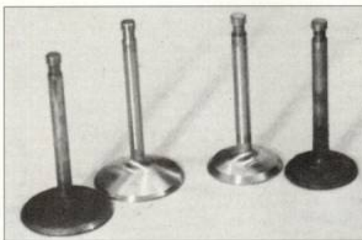
Manley stainless steel valves are lighter, stronger and better flowing than the stock units. The Manleys are the silver ones; the others are stock valves.
