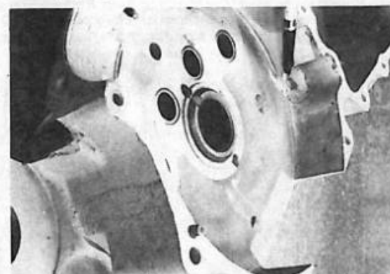
10. This right crankcase half was modified at the Harley factory during prototype development. The pen points to a weld plugging the breather duct.
