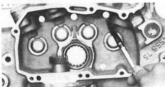
4. Three vent holes (one is indicated by the pen) permit an oil mist to lubricate the cams and gears in the cam case.
