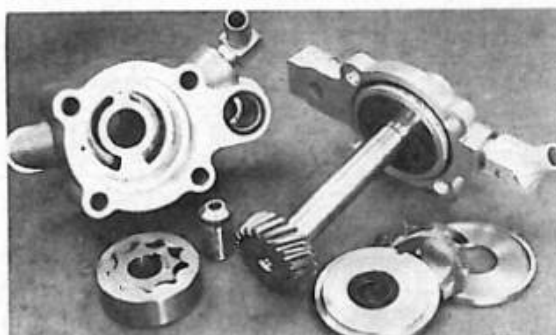
7. Components of the pump reveal that it is a well built precision assembly. It was designed to outlive the early gear pump.
