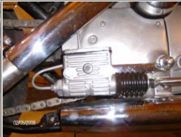
Newer rear brake master cylinder. 14)
