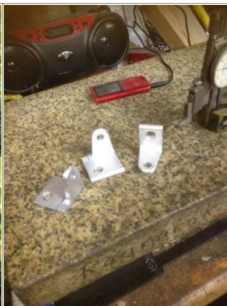
Fabricate some 1/2" 6061 aluminum brackets 3)
