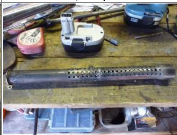
Holes in the baffle partially drilled out. 24)
