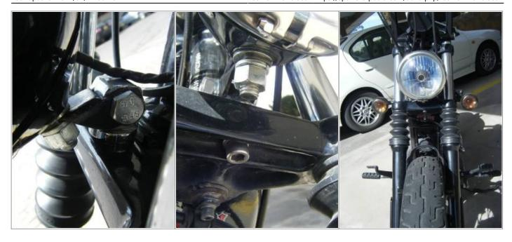
The 2 piece mounts were welded together with a mig welder using flux core wire. Here are some drawings of the mounting bracket (dimensions not to scale). 3)
