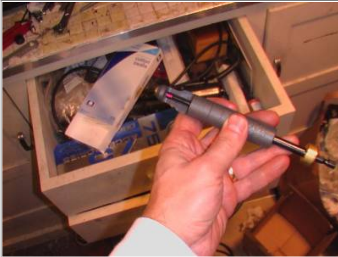
Install the helicoil with the insertion tool 7)
