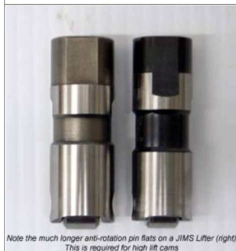
Stock vs Jims lifter tappet flat comparison. 19)
