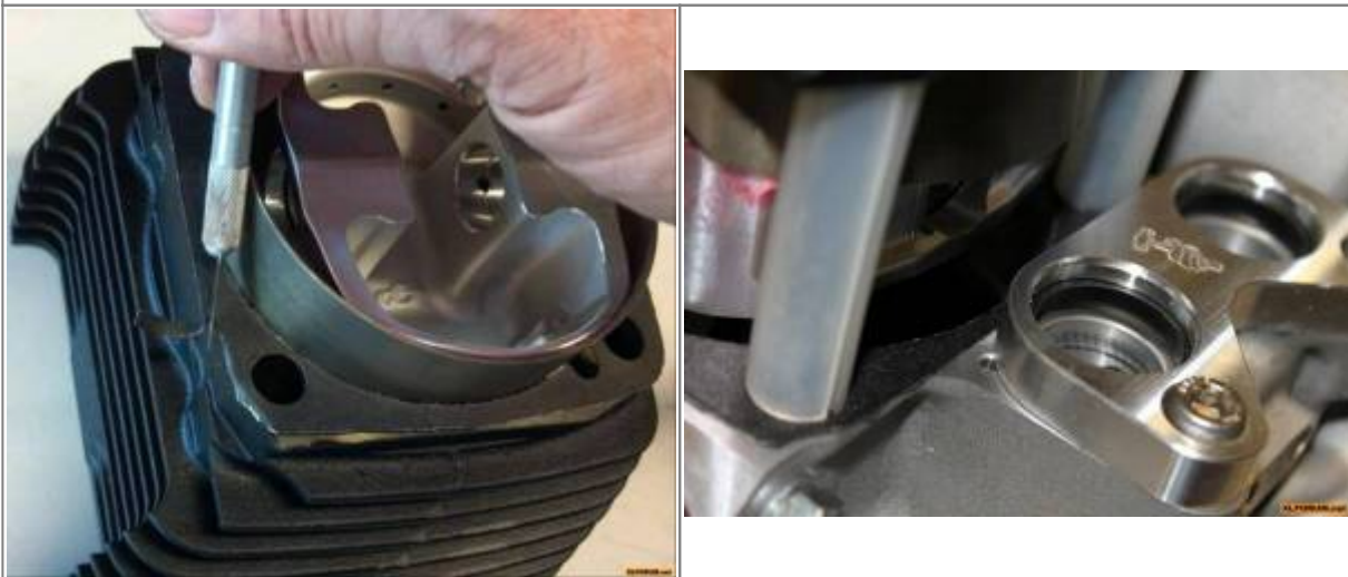
Trimming the base gasket. 16)
