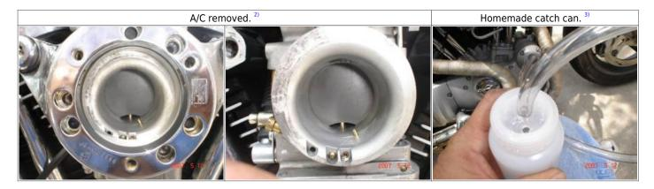
The A/C was re-installed with the venting ran to the catch can.
