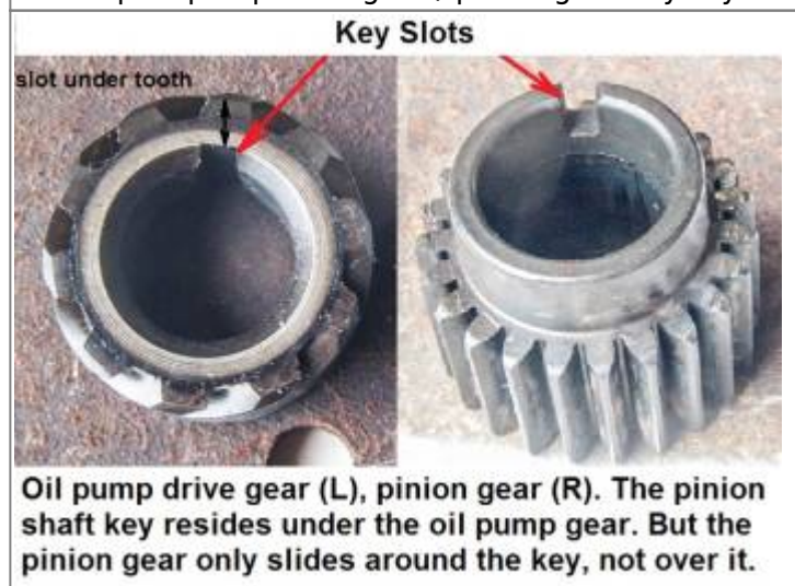
Pinion gear slot aligned with pump gear face. 22)
