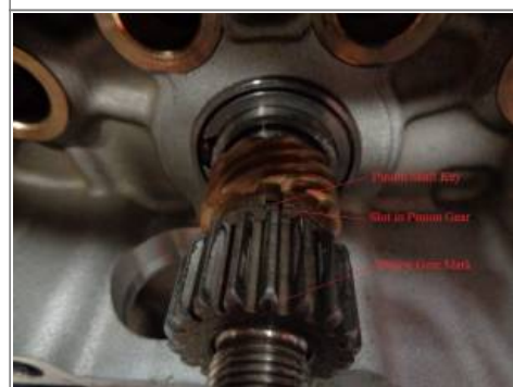
Pinion gear slot aligned with pump gear face. 22)
