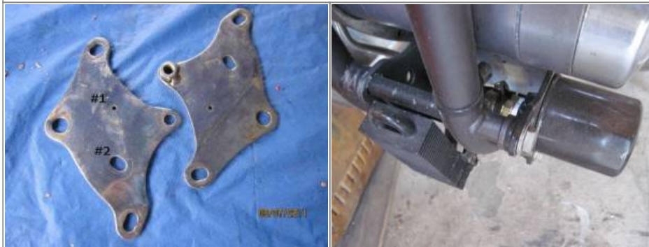
Standard motor mount mod for addition of an oil filter 39)
