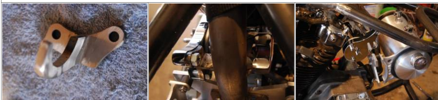
Custom built oil filter mount. 31)
