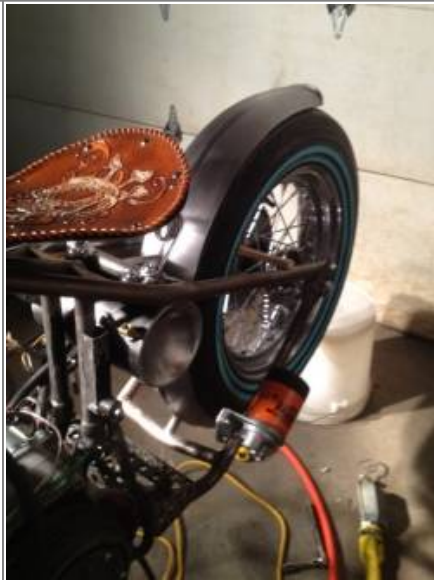
Custom oil filter mount on an 81 XLH 34)
