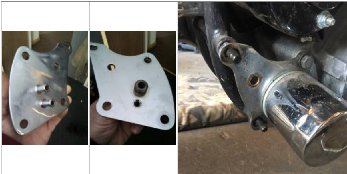
Motor mount oil filter on 69 XLCH 23)
