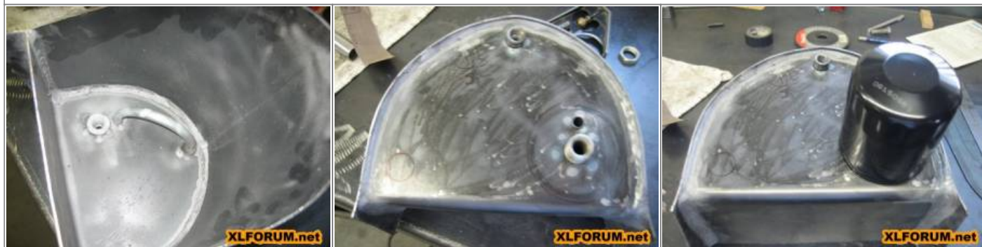
Filter mounted onto oil tank. The return oil goes through a loop inside of tank, back out through filter and returns through center of filter. 37)
