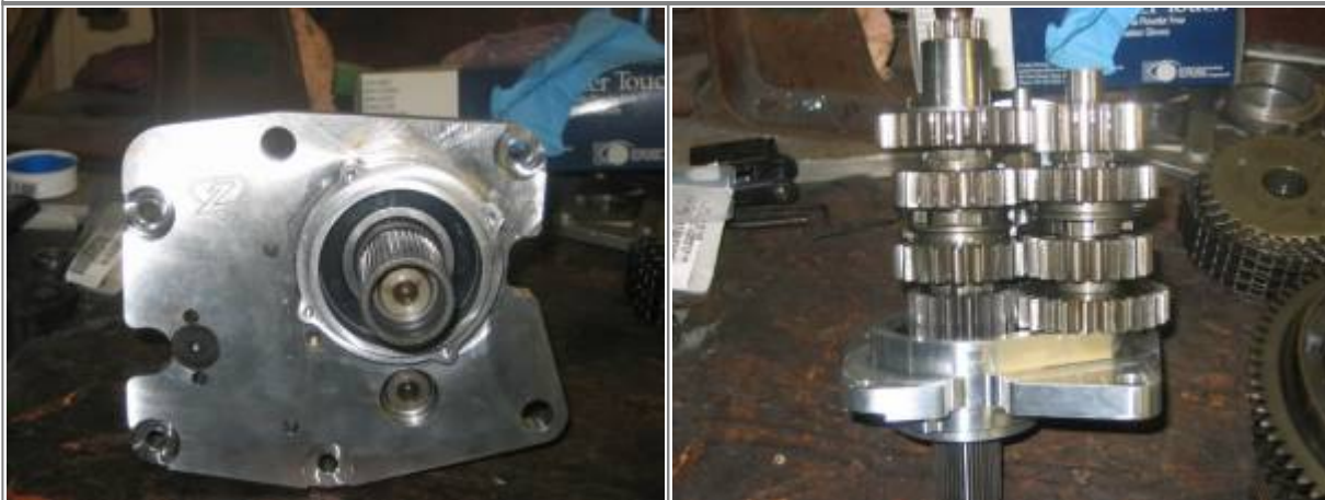
Zipper's Billet Trapdoor w / double row bearings. 31)
