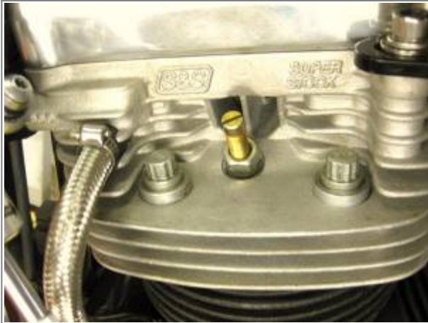
Commercial Piston Stop Installed 6)
