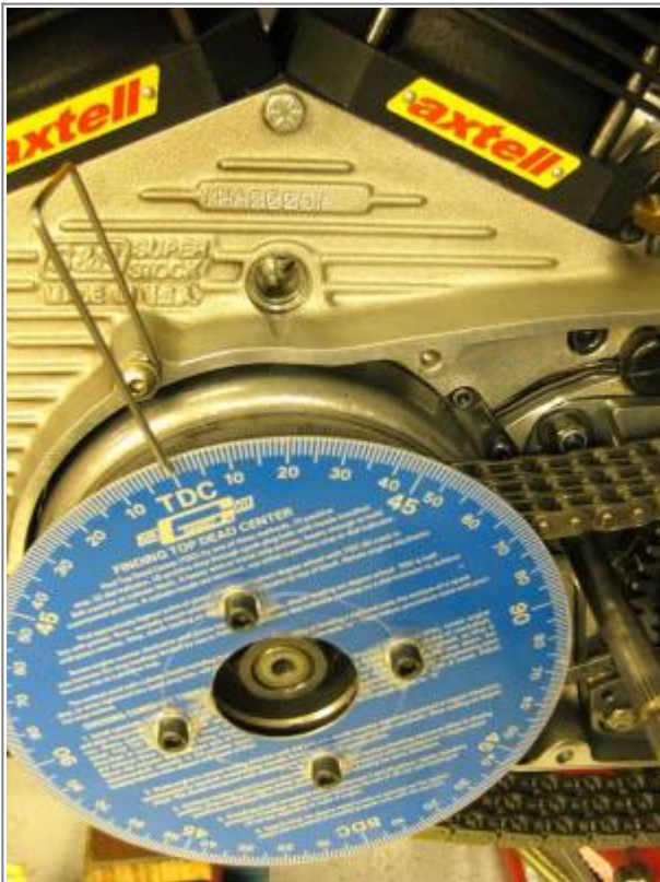
Degree wheel mounted on primary side 7)
