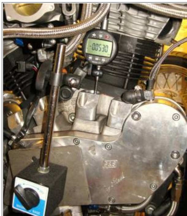
Dial caliper mounted over lifter bore 5)
