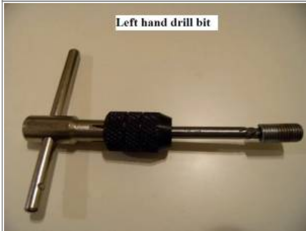
Left hand drill bit for broken bolt removal. 48)
