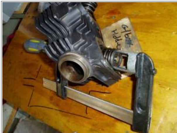
Homemade valve spring compressor, a G clamp and a pipe fitting with a slot hacksawed into it. 4)
