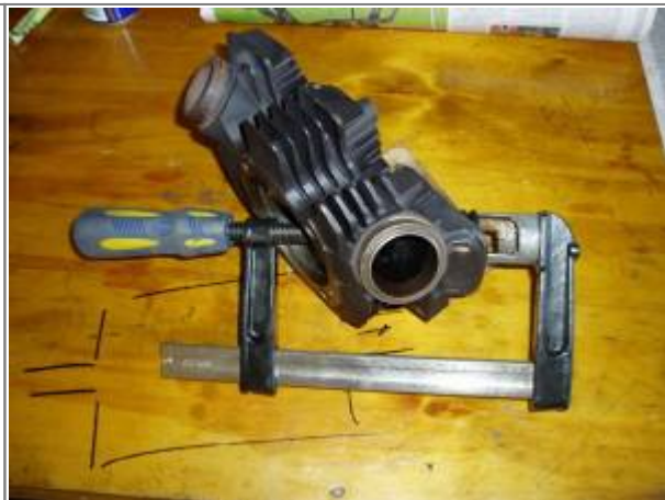
Homemade valve spring compressor, a G clamp and a pipe fitting with a slot hacksawed into it. 4)
