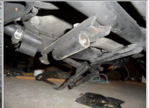
Homemade locking hand lift made one out of scrap and it doesn't need tie-downs. This makes the bike stable enough to sit on, work on and even have both wheels off at the same time. 12)
