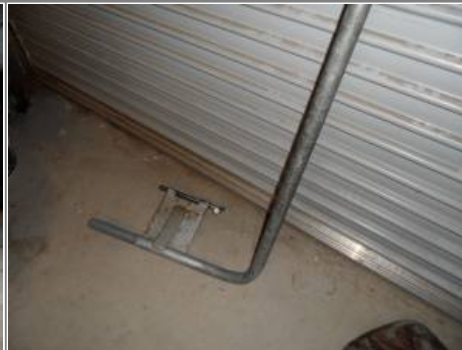
Homemade locking hand lift made one out of scrap and it doesn't need tie-downs. This makes the bike stable enough to sit on, work on and even have both wheels off at the same time. 12)
