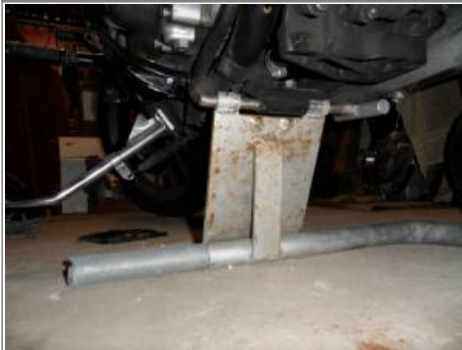
Homemade locking hand lift made one out of scrap and it doesn't need tie-downs. This makes the bike stable enough to sit on, work on and even have both wheels off at the same time. 12)
