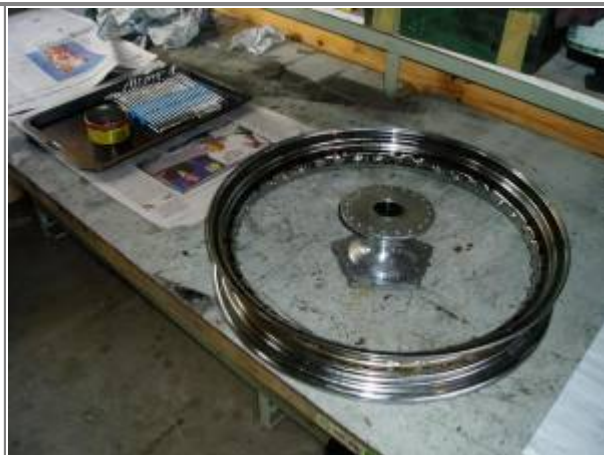
For lacing: To get the initial spoking nice and centered, drill a hole on your work bench for the axle, scribe a circle where the rim goes and locate it with wooden blocks screwed to the bench. Wooden shims provide the correct offset. 3)
