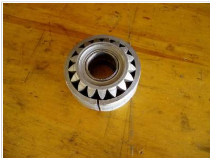
Countershaft low gear bushing jig for use in a 3 jaw chuck lathe 4)
