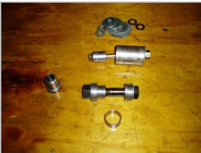
A pair of sockets and a 3/8" bolt for extraction, a stepped collar on a 9/16 bolt to install. 5)
