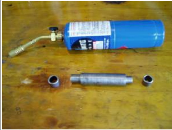
Drift for the transmission countershaft needle roller bearings 7)
