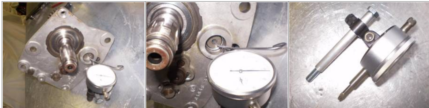
Dial Indicator for checking Countershaft Endplay 2)
