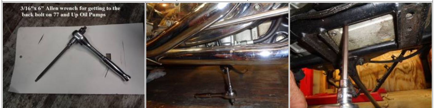
Oil pump removal on 98 and up models. 8)
