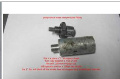
Oil pump check valve tester / pump prelube tool. 6)
