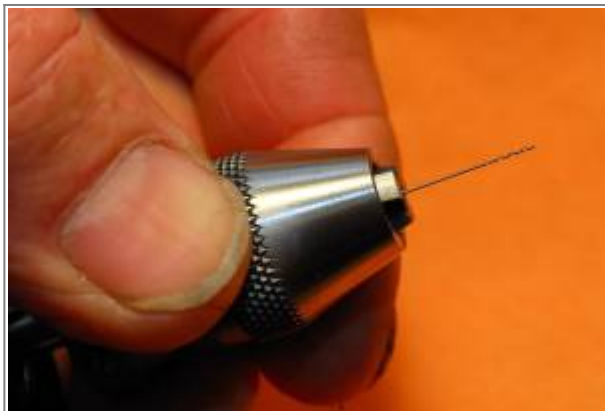
Pin vise made to fit into a regular drill chuck 4)
