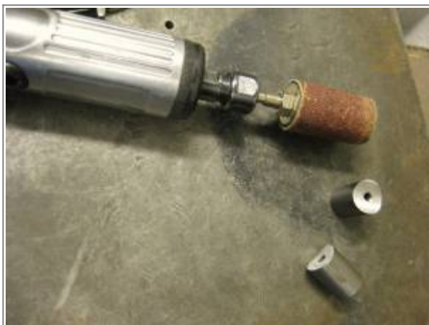
Die grinder used to put a curve in the end of a fabbed frame bung. 5)
