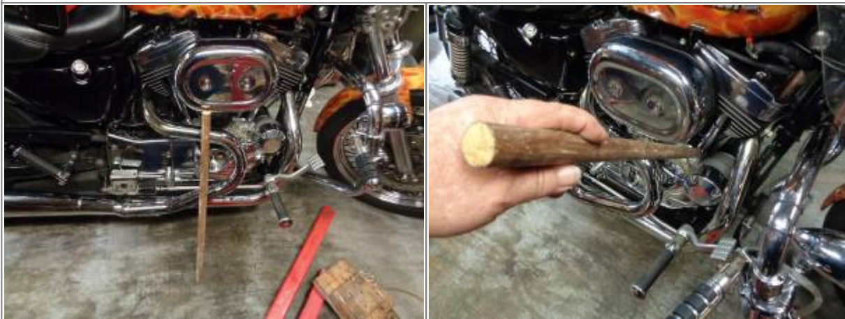
A wooden dowel for a listening tool. 3)
