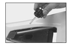
The oil tank drain hose plug is secured to a frame retaining loop. Compress the clamp to pull the hose free of the plug. Then direct it into a drain container.
