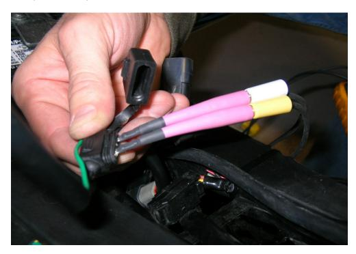
3. With the ignition switch and the accessory switch in the "ON" positions, turn on the seat. If the circuit is working, the current draw should read 2.50-3.50 amps.
