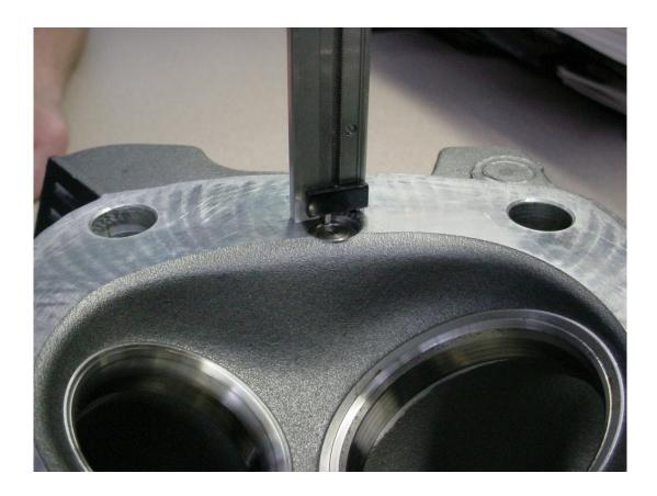
If the automatic compression release is more than .090" from the surface of the cylinder head dome, the component should be removed from the head, cleaned and reinstalled using the ACR socket tool (Part Number **HD-48498A**)
