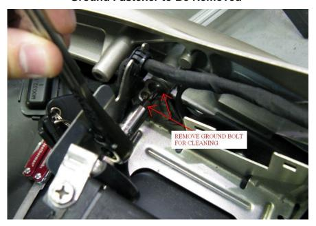
Once the faster is removed, lightly sand both the threads and the face of the screw. (See image below)
