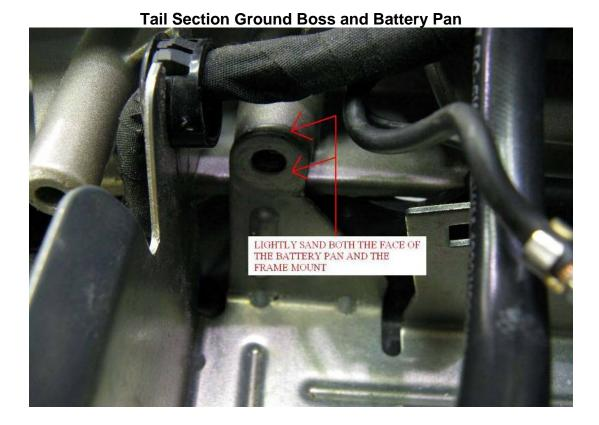
After all of these surfaces have been cleaned, apply dielectric grease to the fastener and reinstall to 72-108 in/lbs.  $(97.6-146.4\ Nm)$ .
