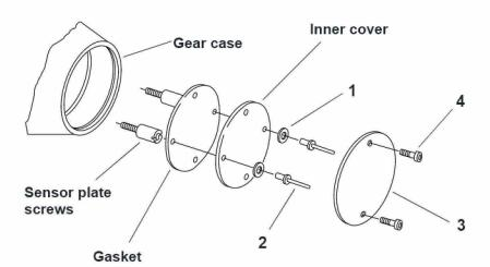
Item Description Part No. ltem Description Part No. 6335 94555-97 1 Washers (2) 4 Timer cover screws (2) 2 5 8501 Rivets (2) Self-tapping screw (not shown) 3659 3 Timer cover not sold separately
