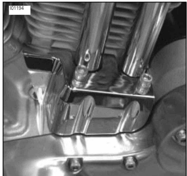
Figure 2. Installed tappet block cover
