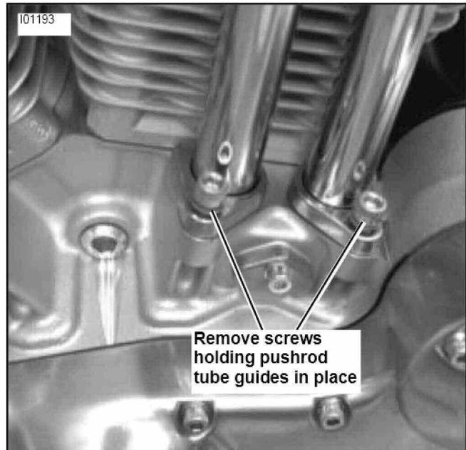
Figure 1. Remove screws
