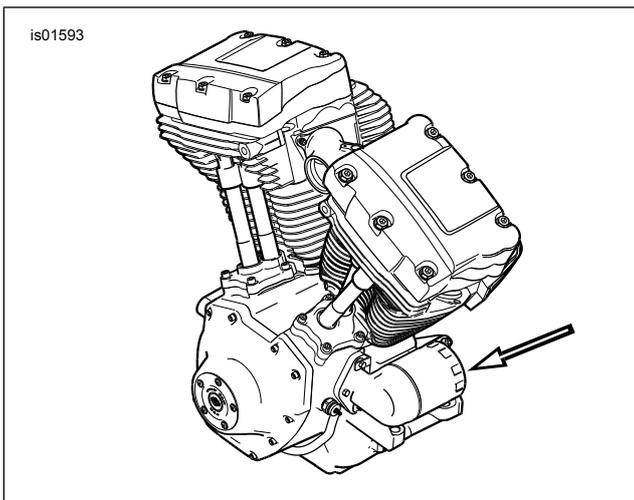
**Figure 2. Spin-On Oil Filter (Twin Cam Engine)**
