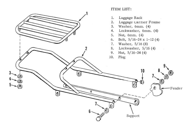
Attach luggage rack (1) to luggage carrier frame (2) using four flat washers (3), lockwashers (4) and nuts (5).
