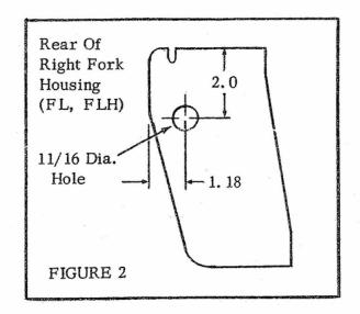
panel. Locate, centerpunch and cut or drill 11/16 in. dia. hole as shown in Figure 3. Install lamp assembly on panel as shown in Figure 1. Reinstall panel and attach lamp wire terminal to terminal No. 21 of fork terminal plate.
