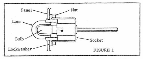
Assemble lamp parts as shown above on all models. If this lamp is installed on motorcycles with 6 volt electrical system, remove bulb and substitute 6 volt bulb, part No. 71090-47 (Trade No. 44). Fiber washer supplied with lamp parts is not used and should be discarded.
